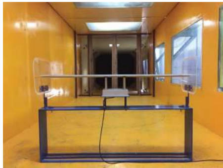
Figure 10. Aerodynamic admittance function identification test.
