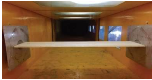
Figure 8. Three-component force test of sectional model.
