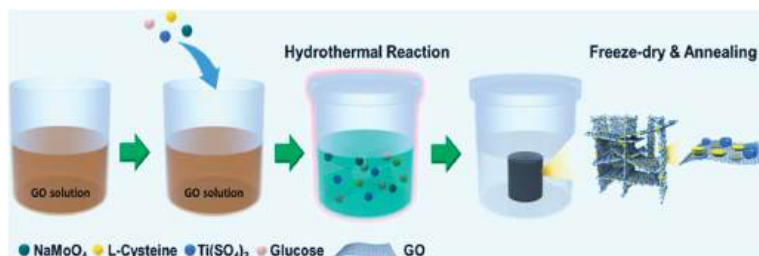
Figure 14. Schematization of one-pot solvothermal synthesis of \text{TiO}_2 -graphene- \text{MoS}_2 composite [165].
