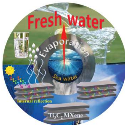
Figure 1. Schematic representation of seawater to freshwater generation by the 2D layer structured \text{Ti}_3\text{C}_2 MXenes.
