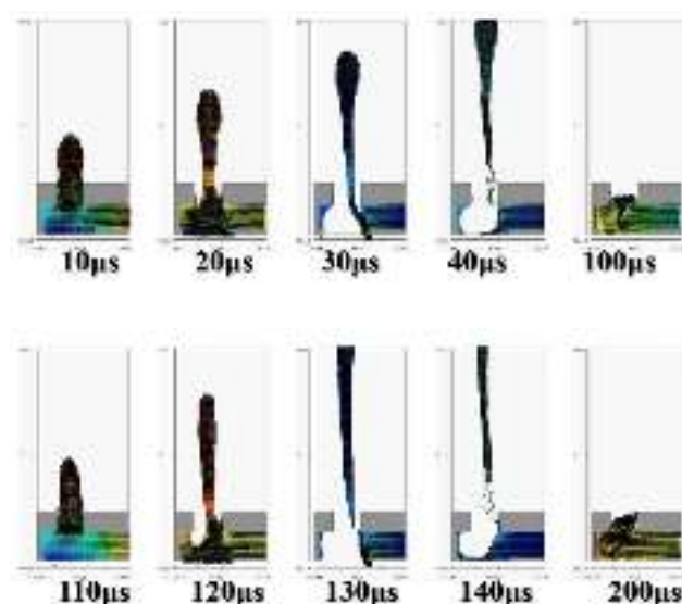
Figure 5. Calculate and simulate water in a single-channel jet cavity with a nozzle diameter of 60 \mu\text{m} and a thickness of 50 \mu\text{m} , with an operating frequency of 10 KHz, in the XZ two-dimensional cross-sectional view, at 10, 20, 30, 40, 100, 110, 120, 130, 140 and 200 \mu\text{s} injection situation.
