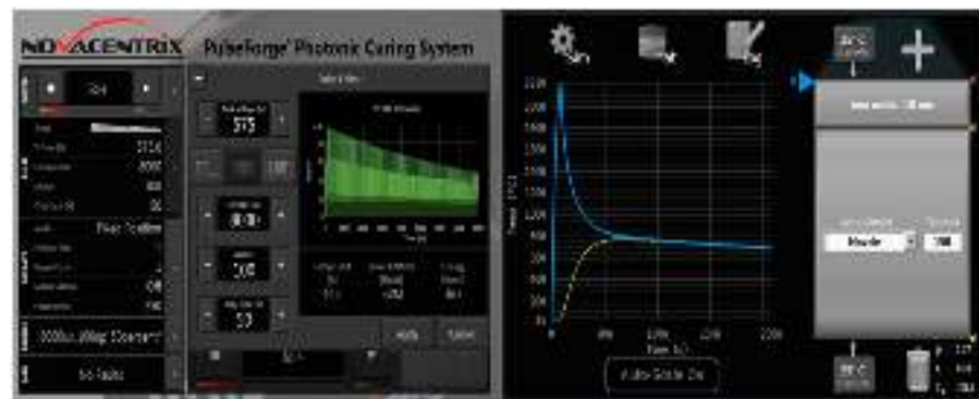
Figure 3. (Left) Screenshot of an example pulse sequence used on the PulseForge® 1300 to photosinter strontium ferrite thin films. (Right) SimPulse® predicted temperature profile for the pulse indicated.
