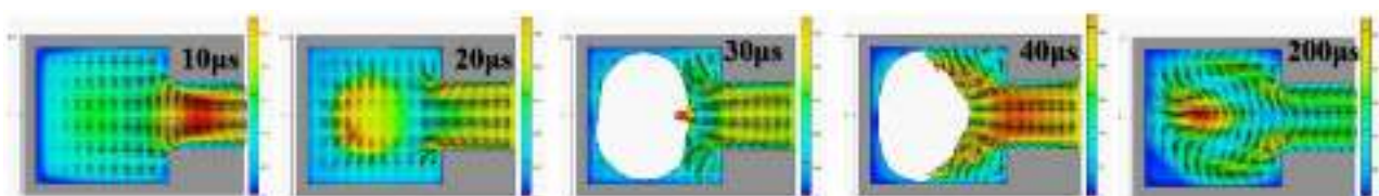
Figure 4. Calculate and simulate the injection of water in a single-channel injection chamber with a nozzle diameter of 60\text{ }\mu\text{m} and a thickness of 50\text{ }\mu\text{m} , at an operating frequency of 5\text{ KHz} , in the X-Y two-dimensional cross-sectional view, at 10 , 20 , 30 , 40 and 200\text{ }\mu\text{s} .
