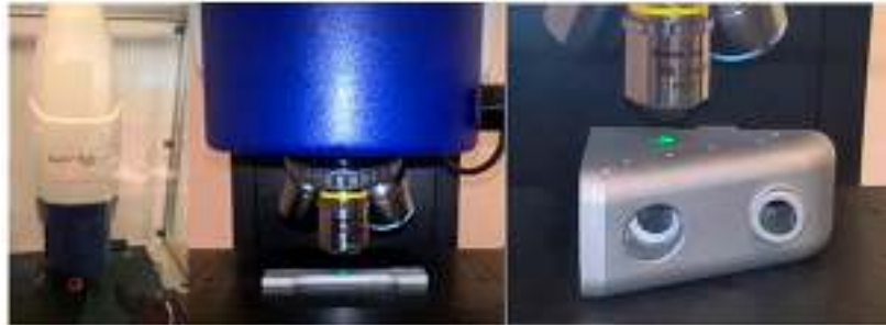
Figure 3. Talysurf CCI Lite—optical profilometer, samples during measurements.
