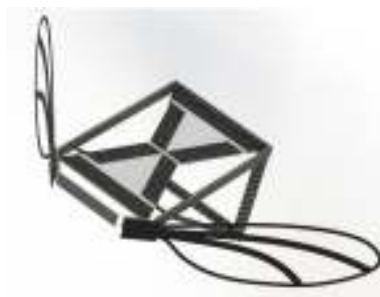
Figure 5. Concept design of a micro aerial vehicle, composed of MEMS and 3D-printed parts. Reproduced with permission from [77].
