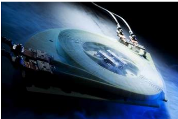
Figure 9.1.3: 2G coated conductor fault current limiting element (Photo: KIT)
