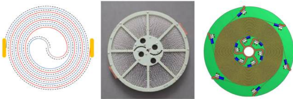
Figure 4.3.1: Schematic diagram of a bifilar coil (left) and a designed current limiter module with high-temperature superconductors [Kraemer2021] (middle). On the right a multifilar arrangement with three bifilar coils in parallel [Noe2012]
