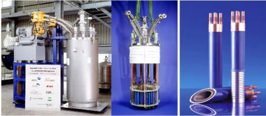
Figure 9.1.2: 10 kV, 600 A CURL10 fault current limiter (left) and Bi2212 bulk material current limiting element (right) [Bock2005, Kreutz2005]
