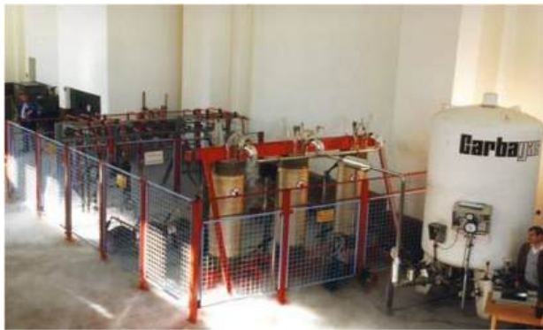
Figure 9.1.1: 10 kV, 70 A shielded core type superconducting fault current limiter from ABB [Paul1997]
