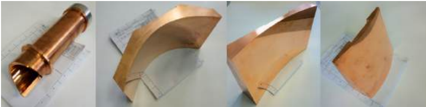
Fig. 3.30: Pictures of the manufactured quasi-optical output coupler. Launcher, quasi-elliptical and two beam shaping mirrors from left to right are depicted.
