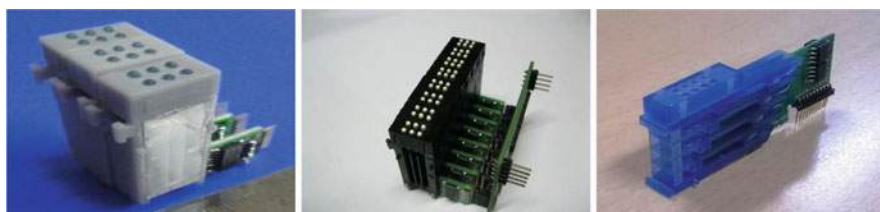
Fig. 5.10 Initial single Braille cell based on SMA (Shape memory alloys) designed and fabricated during 2014–2017
