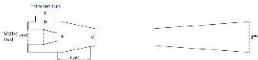
Figure 12. Spray ejector condenser 1^{\text{SEC}} : Nozzle inlet, a: Nozzle outlet, a–c: Mixing chamber, b: Suction chamber, c: Throat (part of Diffuser), c-2 ^{\text{SEC}} : Diffuser, 5 Inlet of entrained fluid, 5-MC: Entrained fluid in mixing chamber.
