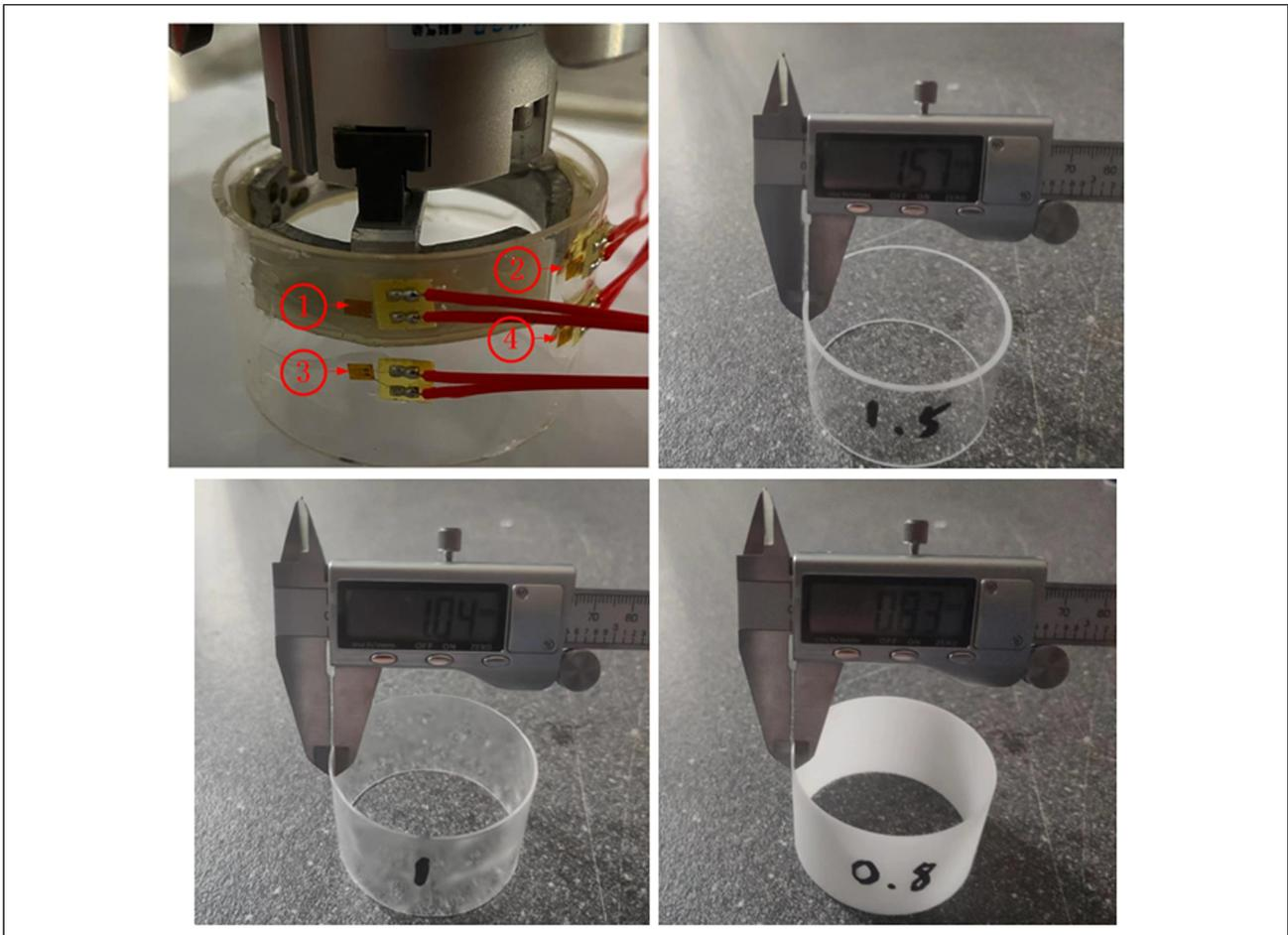
**Figure 22.** Thin wall glass ring and strain gauge pasting.
