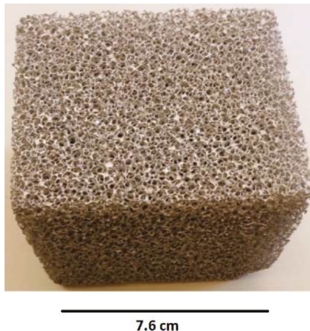
Figure 1. Photograph of a block of open-cell aluminum foam with 20 pores per inch. (Photo taken by author).
