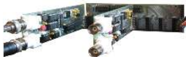
Figure 3. Hot-wire anemometer with automatically adjusted dynamic properties.
