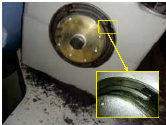
Figure 10. Main bearing offset failure.
