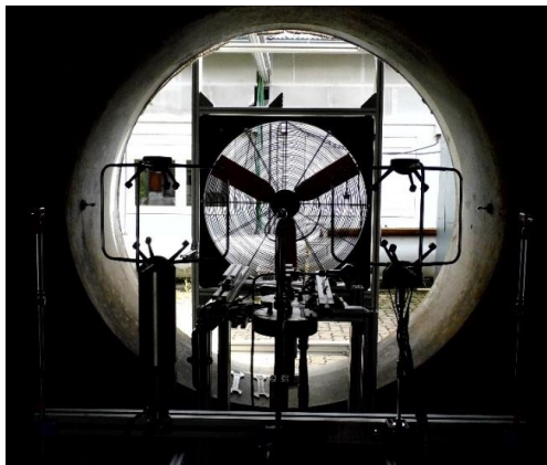
Figure 1: b View from downstream on the ventilated tunnel segment with central fan
