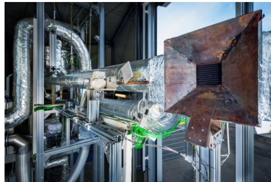
Figure 3: The thermal receiver of the SOMMER test facility with copper shield (Foto: Amadeus Bramsiepe/KIT)
