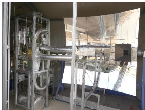
Figure 5: SOMMER test facility; left: parabolic mirror; right: liquid metal loop with thermal receiver in the focal point (Foto: F. Fellmoser)
