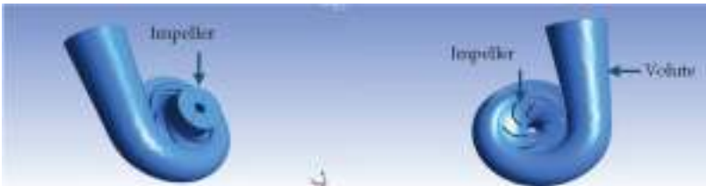
Figure 8. Side views of the pump designed in Vista CPD.
