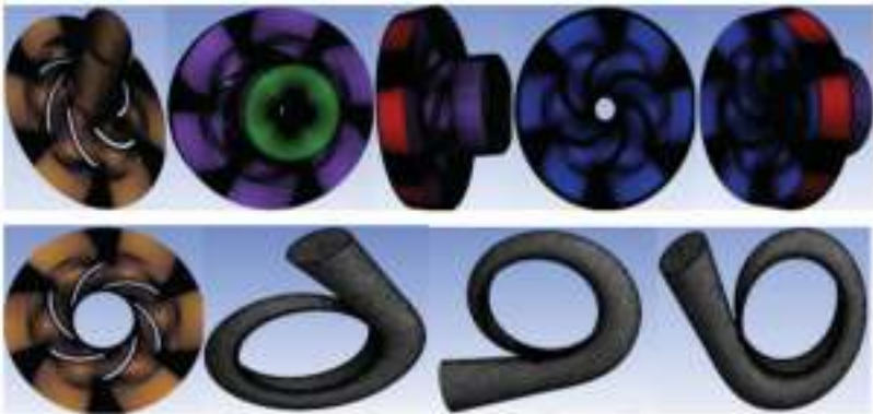
Figure 9. Meshing of the impeller and volute.
