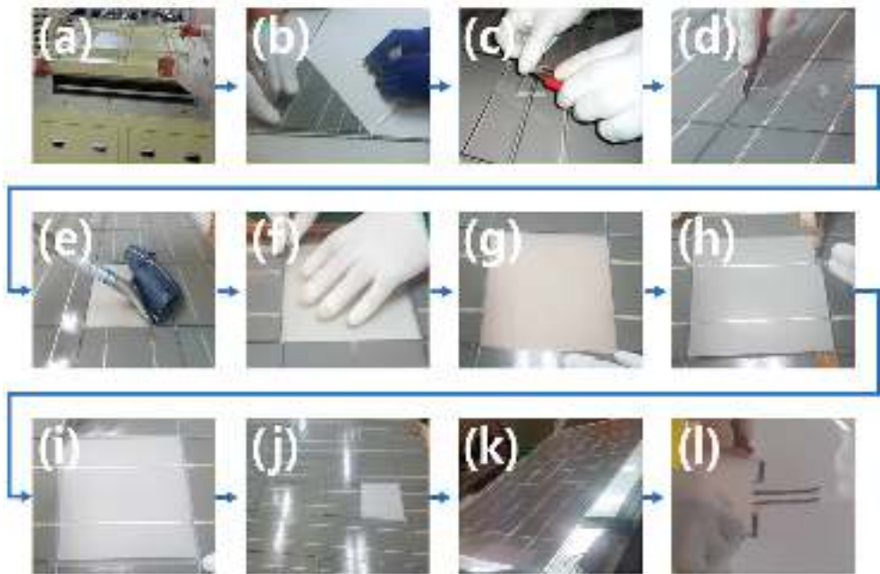
Figure 3. Module recovery process by replacing broken cells. (d) Next, the EVA along the boundary of the cell to be removed was cut, and the tab of the cell to be removed was cut by 15 mm or more for electrical connection during recovery. (e) Subsequently, the broken cell was removed using a scraper with a blade. (f) The remaining EVA was trimmed to the interface of the adjacent cells, and the removed surface was washed. After cell removal, the module was removed from the hot plate and cooled to room temperature. (g) EVA was placed between the glass and the new cell to connect it to the module. Here, the size of the EVA is important because it should be perfectly connected to the first EVA of the existing module without leaving a bubble after lamination of the module. Thus, the EVA should be cut accurately with an error of less than 1 mm. If it is larger than the removal surface, stress is applied to the replacement cell, which can cause the cell edge to crack during the lamination process. (h) Subsequently, while electrically connecting the new cell and the existing adjacent cell through re-soldering, insulation was applied to prevent the first EVA from melting in the heat. (i) The second EVA was slightly thicker than the original size. (j) A margin of less than 5 mm should be given, and if it is more than that, the overlapping part of the edge EVA of the cell replaced after lamination is exposed, causing a repair mark. (k) Finally, the EVA and new back sheet covering the entire module were laid up. (l) The electrical connection was checked, and the lamination process was completed.
