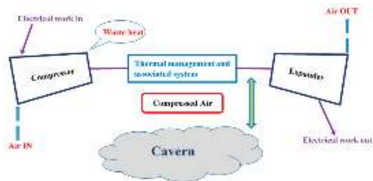
Figure 3. Compressed air energy storage system schematic.
