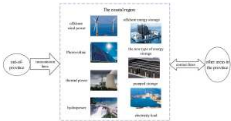
Figure 3. Power supply and line structure in this coastal area.
