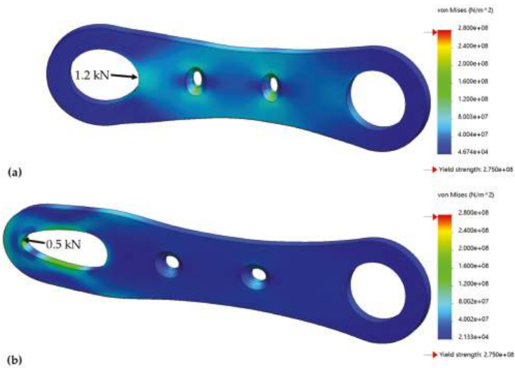
Figure 16. Stress analysis of the connecting rod elements in (a) compression and (b) tension.
