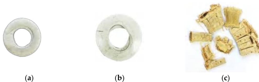
Figure 6. Shape of tube after deformation: (a) PVC Ø 20 (b) PVC Ø 25 and (c) Bamboo.
