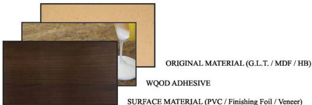
Figure 3. Material composition of the test piece.
