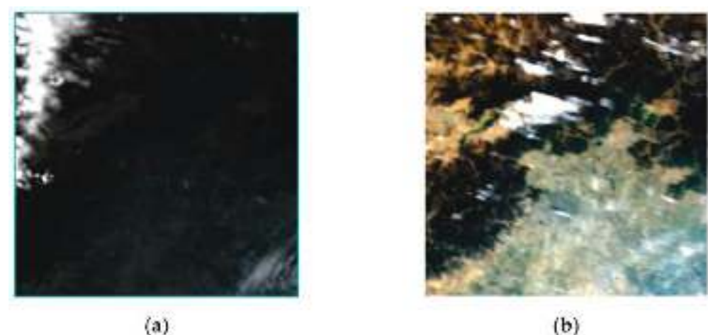
Figure 4. (a) is the satellite image with full channel information, and (b) is the synthesized RGB image.
