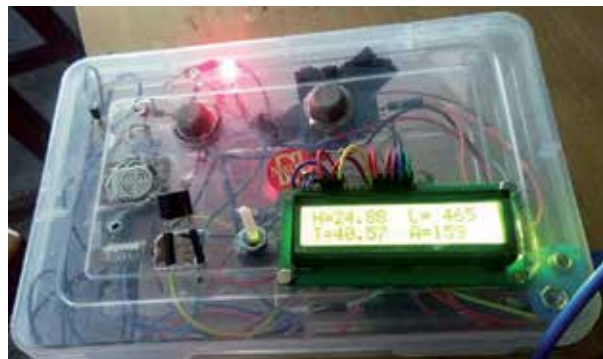
Figure 4. Actual readings of each sensor on LCD.
