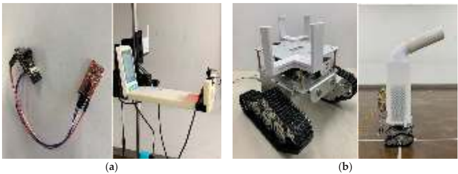
Figure 7. Data communication module and remote transfer unit used in the experiment: (a) Data communication module, (b) Remote transfer unit.
