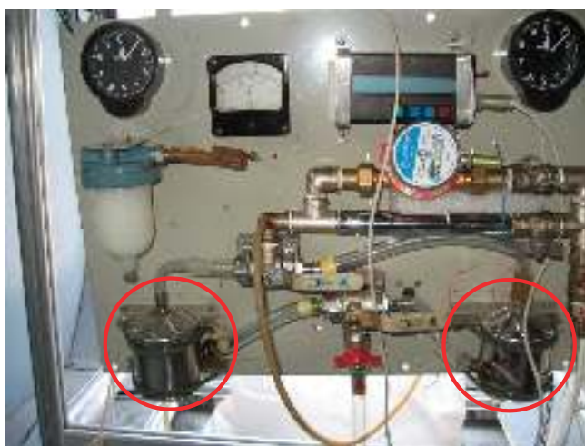
Figure 4. Photo of two impingers (red circles) at a sampling stand of microorganisms located in atmospheric aerosol.
