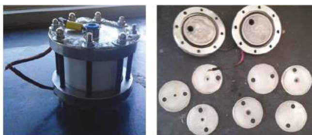
Figure 3. Electrolyser (left) and, steel electrodes used in the electrolyser unit (right).
