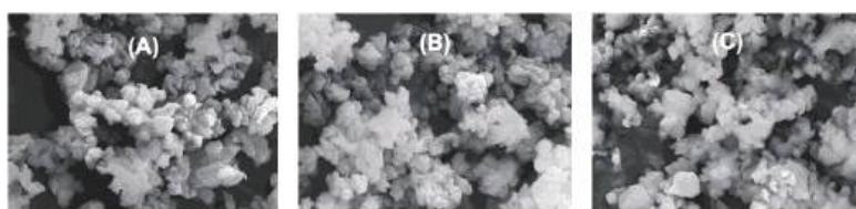
Figure 2. SEM images (5000×, 1 \mu\text{m} ) of shell mix solid catalyst, (a) before calcination, (b) after calcination, and (c) after the first transesterification step.
