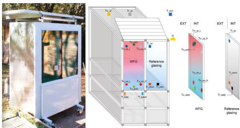
Figure 7. Set up of the Spanish mock-up and schematic of sensors distribution of the cabins. Sensors nomenclature and position for the WFG cabin and the Reference cabin.
