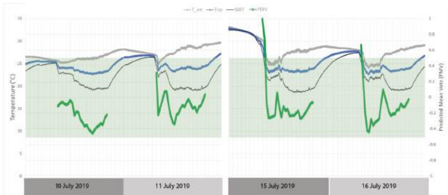
Figure 16. Operative temperature ( T_{op} ) and Predicted Mean Vote (PMV) in summer—sample days 10 July 2019 to 11 July 2019 and 15 July 2019 to 16 July 2019.
