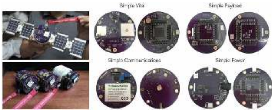
Figure 7. Low-cost sensing solution from SimpleSpace. The simple unit is divided in subsystems which can be adapted into a vertical bus which allows the insertion of new pcb layers with new measurement instruments.
