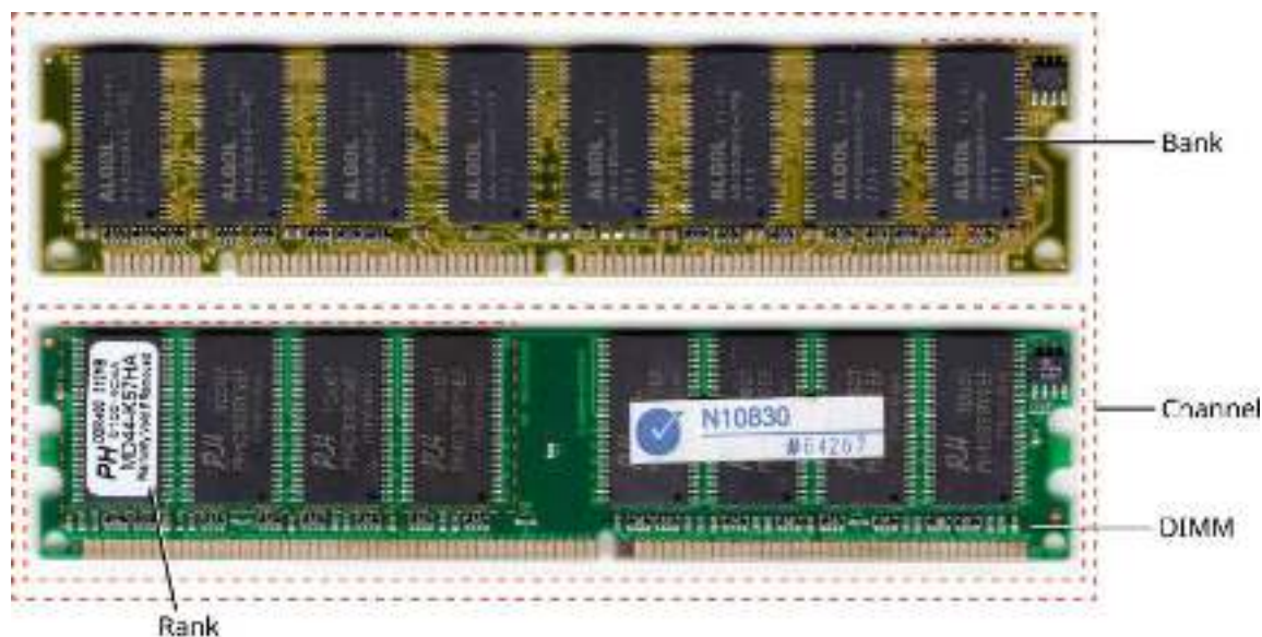
Figure 5.22 DRAM memory banks can be organized into chips, ranks, DIMMs, and channels. (credit: modification of "168 pin and 184 pin DIMM memory modules" by Veeblefretzer/Wikimedia Commons, CC BY 4.0)
