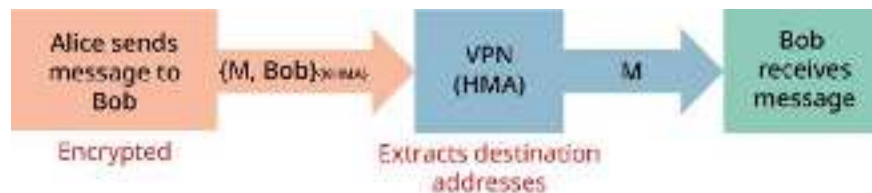
Figure 14.10 When Alice sends a message to Bob, HMA accepts encrypted messages, then extracts the corresponding destination addresses and forwards the messages accordingly. (attribution: Copyright Rice University, OpenStax, under CC BY 4.0 license)
