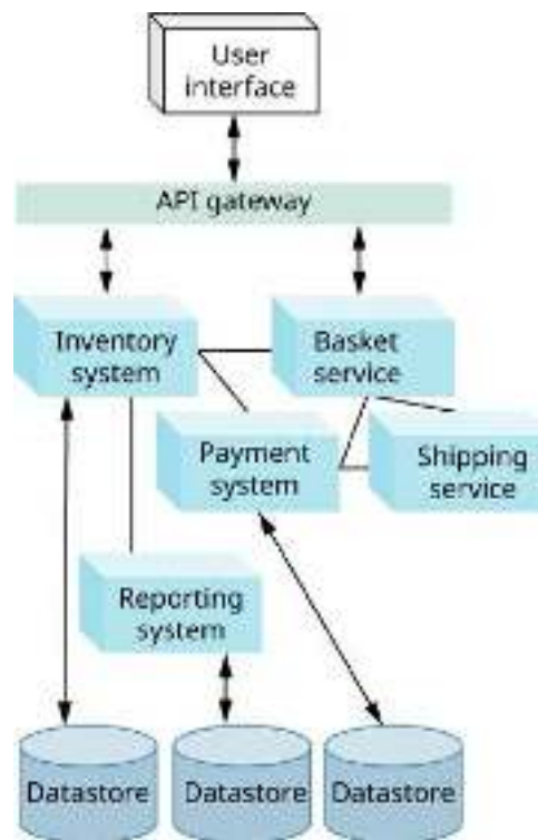
Figure 12.6 An application designed using a microservices architecture. (attribution: Copyright Rice University, OpenStax, under CC BY 4.0 license)
