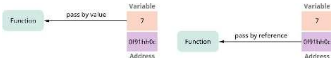
Figure 7.16 Compare passing a parameter by value versus passing it by reference in C++. (attribution: Copyright Rice University, OpenStax, under CC BY 4.0 license)
