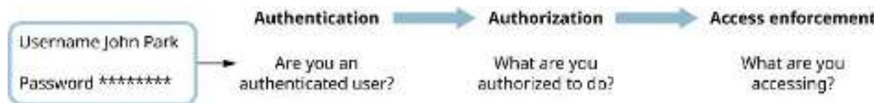
Figure 6.36 The first step of the protection mechanism is authentication, which checks the username and password; then comes authorization, which checks the privileges; and, finally, there is access enforcement, which controls access. (attribution: Copyright Rice University, OpenStax, under CC BY 4.0 license)
