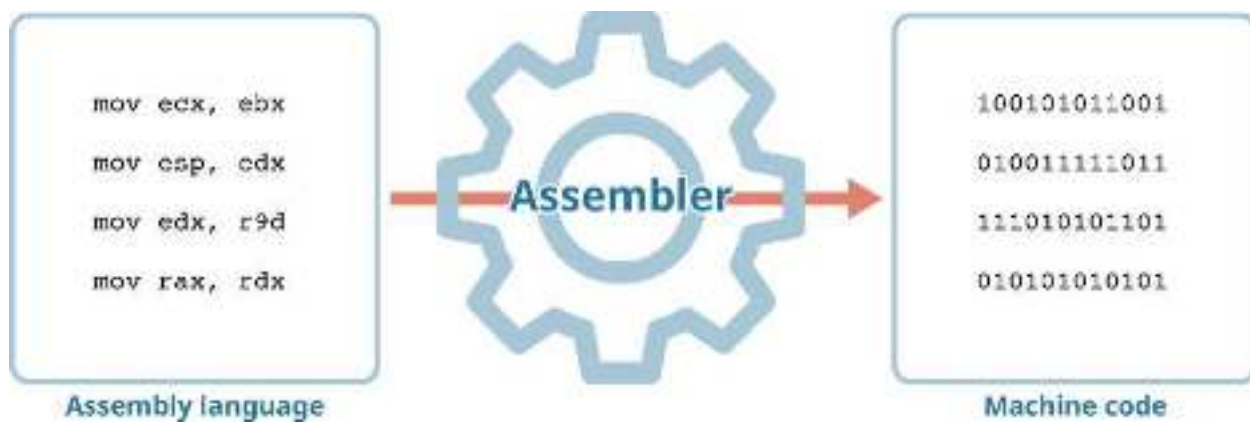
Figure 4.7 An assembler is a program that translates assembly language source code into machine object code. (attribution: Copyright Rice University, OpenStax, under CC BY 4.0 license)
