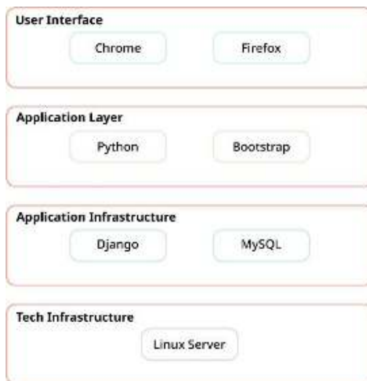
Figure 10.47 The stack consists of a user interface, application layer, application infrastructure, and tech infrastructure. (attribution: Copyright Rice University, OpenStax, under CC BY 4.0 license)
