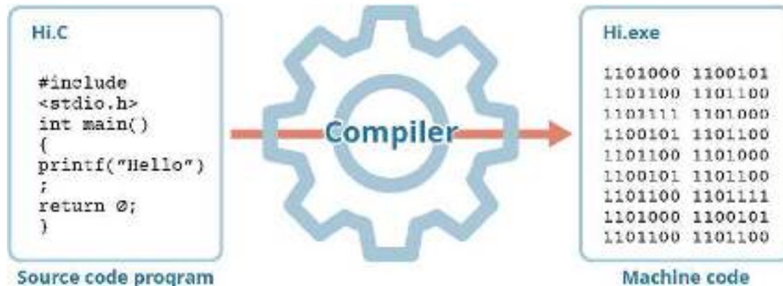
Figure 5.7 A compiler takes code written in an HLL and converts it to “computer-friendly” and simple code called assembly language. (attribution: Copyright Rice University, OpenStax, under CC BY 4.0 license)
