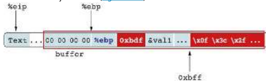
Figure 14.26 Code injection is performed by hijacking the saved %eip and changing it to point to the address of the injected code. (attribution: Copyright Rice University, OpenStax, under CC BY 4.0 license; credit: reproduced with permission from Dave Levin)
