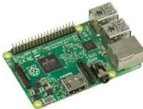
Figure 4.33 A Raspberry Pi demonstrates the concept of a system-on-chip (SOC). (credit: “Raspberry-Pi-2-Bare-BR” by “Evan-Amos”/Wikipedia, Public Domain)
