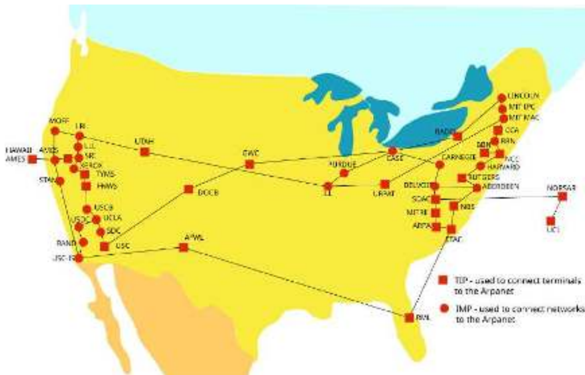
Figure 1.3 The ARPANET, circa 1974, was an early predecessor to the Internet. It allowed computers at Pentagon-funded research facilities to communicate over phone lines. (credit: modification of "Arpanet 1974" by Yngvar/Wikipedia, Public Domain)
