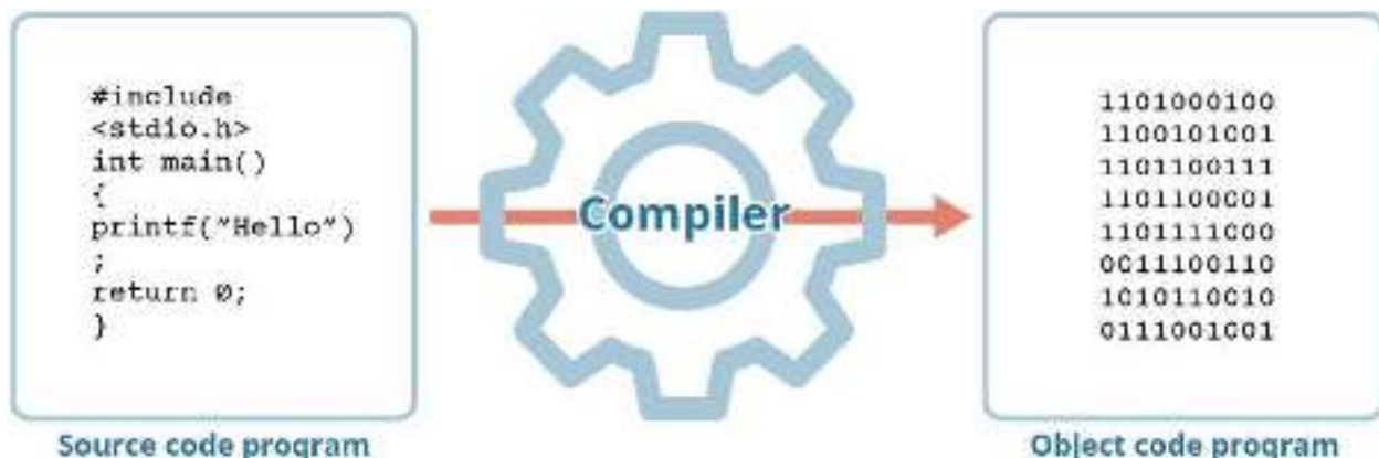
Figure 7.7 A sample C++ source program is compiled into machine language to run on a particular platform. (attribution: Copyright Rice University, OpenStax, under CC BY 4.0 license)
