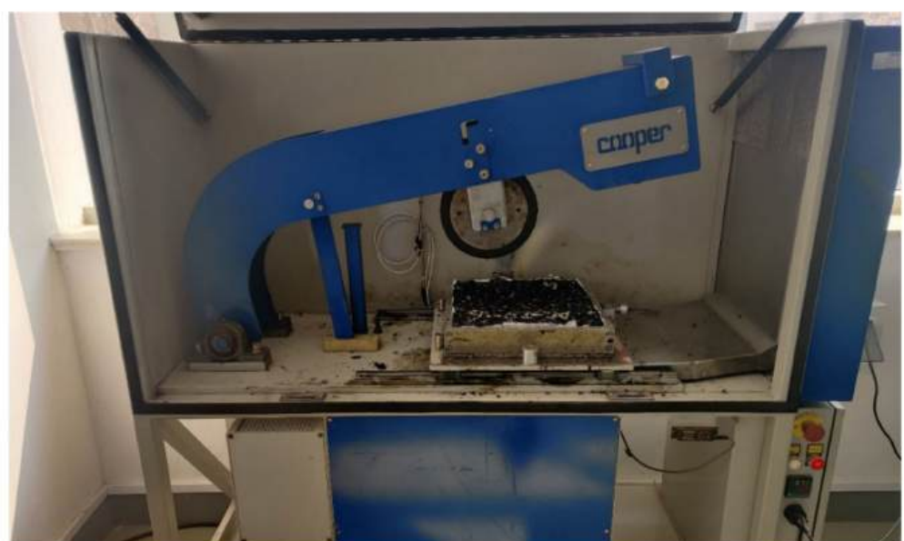
Figure 12. Wheel tracking test.
