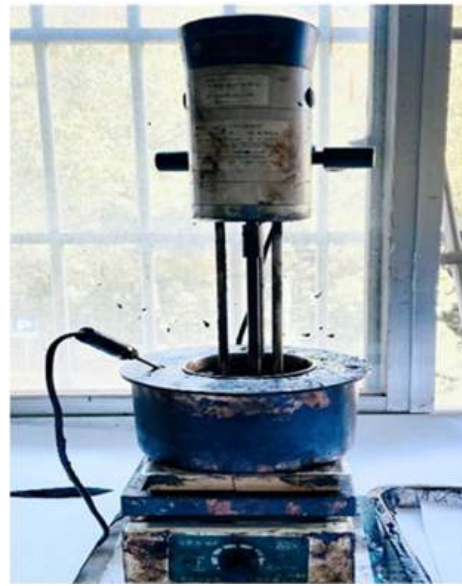
Figure 2. High-speed shear agitator for BRA-MA preparation.
