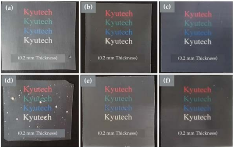
Figure 4. Digital images showing the transparency of (a) PP, (b) PP-8.75 SS, (c) PP-8.75 SP, (d) PP-1.25 CNF, (e) PP-SS/CNF, and (f) PP-SP/CNF.
