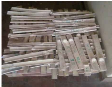
Figure 4. Unplaned bamboo strips produced with the bamboo culm splitter.
