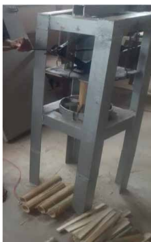
Figure 3. Bamboo culm splitter developed at the University of Ibadan, Nigeria.
