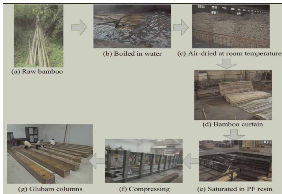
Figure 7. Manufacturing process of Glulam (adapted from [18] with permission).
