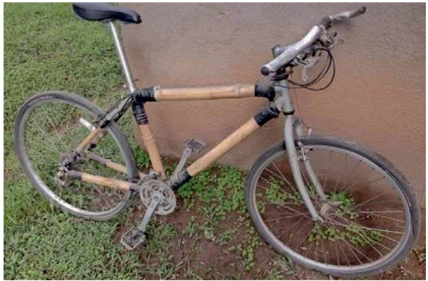
Figure 8. Bamboo bicycle produced at the University of Ibadan, Nigeria.
