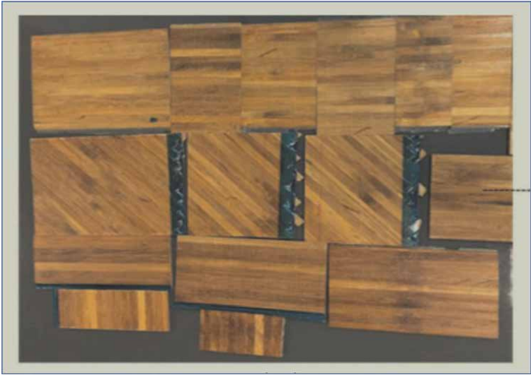
Figure 11. Manufactured bamboo – PLA composite panels (adapted from [36]).
