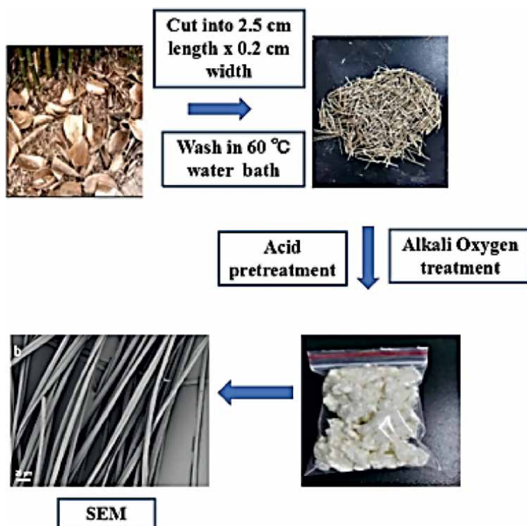
Figure 3. Degumming process of BSSF [29].
