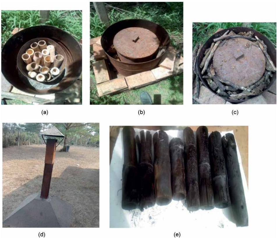
Figure 9. a. the bamboo charcoal kiln with retort open. b. the bamboo charcoal kiln with retort closed. c. the furnace stocked with firewood. d. the bamboo charcoal kiln chimney. e. the bamboo charcoal produced.
