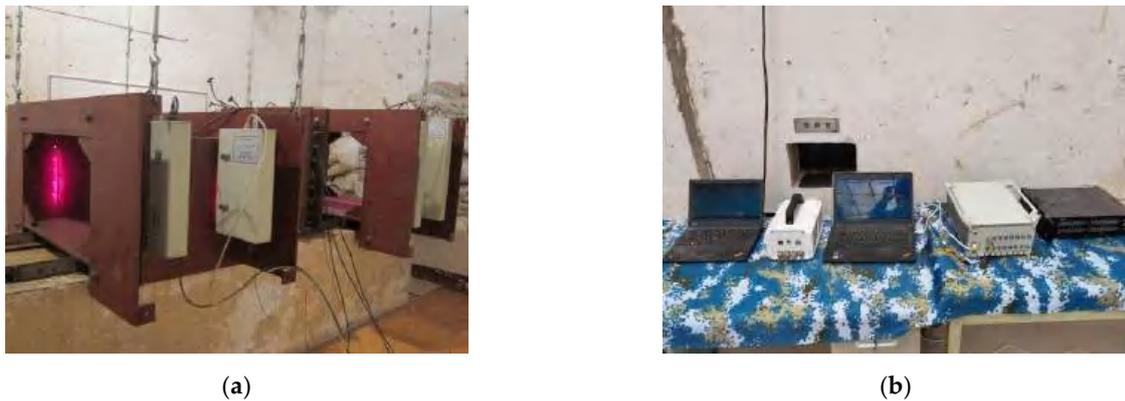
**Figure 2.** Test equipment and recording devices. (a) Laser velocimeter; (b) high-speed camera, pressure sensor and target-net velocimeter.
