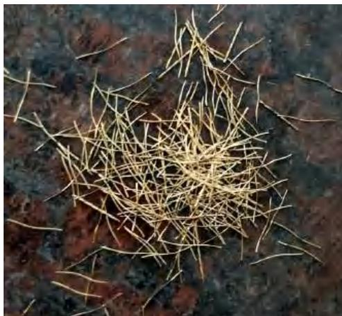
Figure 2. Straight copper-coated steel fibers.
