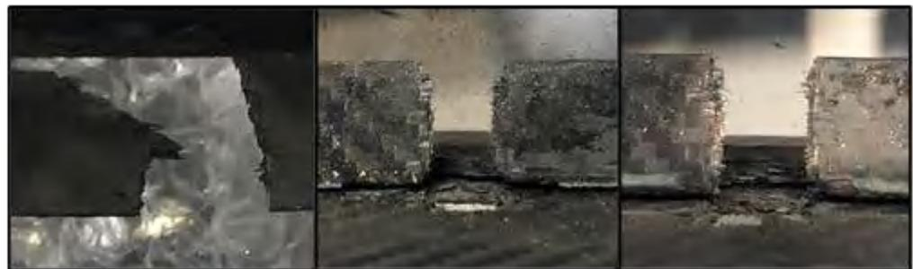
**Figure 10.** Typical damage mode of composite stringer.
