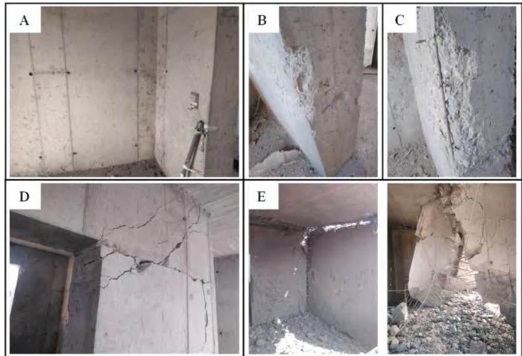
**Figure 13.** Different effects of IEDs on the interior structure: (A) after the two black powder tests (T1–T2); (B) after the ANFO tests (T3–T4); (C) after the AN/AL tests (T5–T6); (D) after the first PG2 test (T7); (E) after the second PG2 test (T8).
