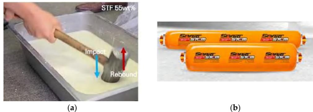
**Figure 4.** (a) Shear thickening fluid-based stemming material image and (b) package products.
