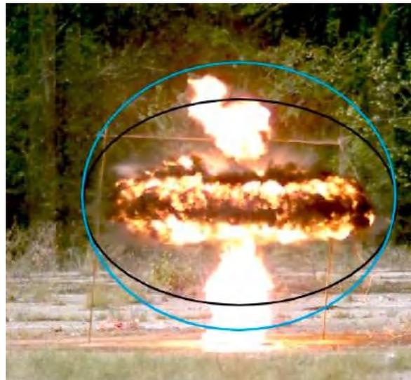
**Figure 8.** Blast wave shape (perfect sphere (blue) and real (black)).
