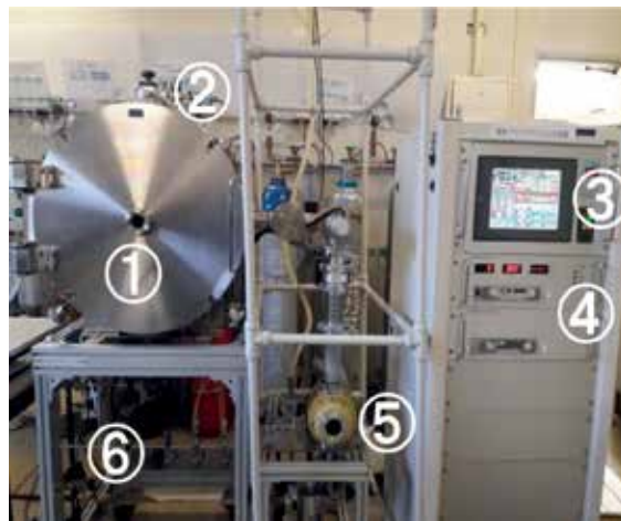
Figure 1. High density RF-DC oxygen plasma etching system. ① vacuum chamber, ② RF-generator, ③ control panel, ④ RF- and DC-power supplies, ⑤ evacuation units, and ⑥ carrier gas supply.
