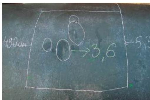
Figure 1. A photograph of corrosion colonies on the steel pipe surface. Author's source.
