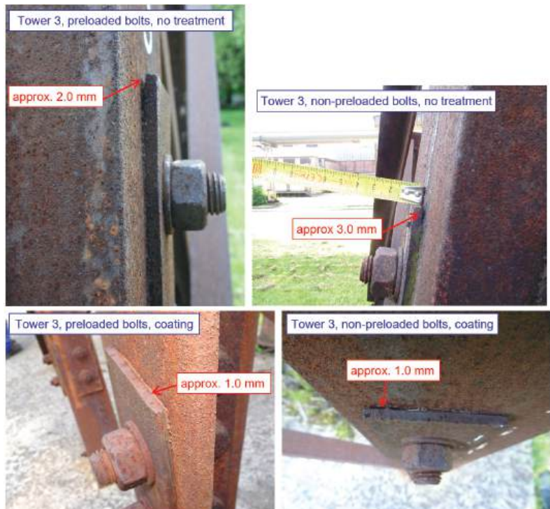
Figure 22. Tower 3: Selected examples of joints (the development of corrosion products in the crevice of joints without treatment, and in joints with coating on the inner surface of the splices).
