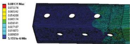
Figure 13. The von Mises equivalent strain in the selected part of the K-type joint (model without the effect of the crevice corrosion).
