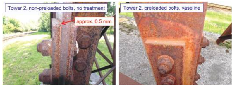
Figure 21. Tower 2: Selected examples of joints ((left): initial development of corrosion products in the crevice; (right): visual influence of the development of corrosion products in the area around the joints protected with Vaseline).
