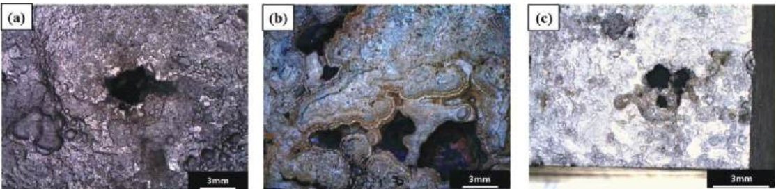
Figure 3. Surface image of the pitting part: (a) pitting corrosion area of the leakage (the outside of the pipe), (b) pitting corrosion area near the leakage (the outside of the pipe), and (c) pitting corrosion area near the leakage (the inside of the pipe).
