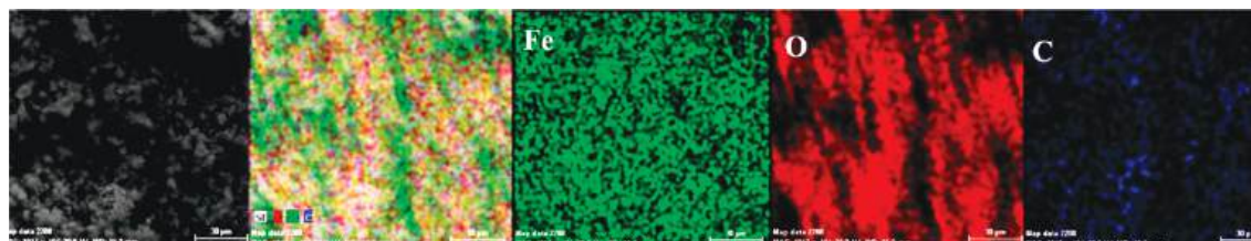
Figure 9. Elemental distribution on the surface of the crust of reaction products in the case of the C45/BSW system, after 85 days of immersion.
