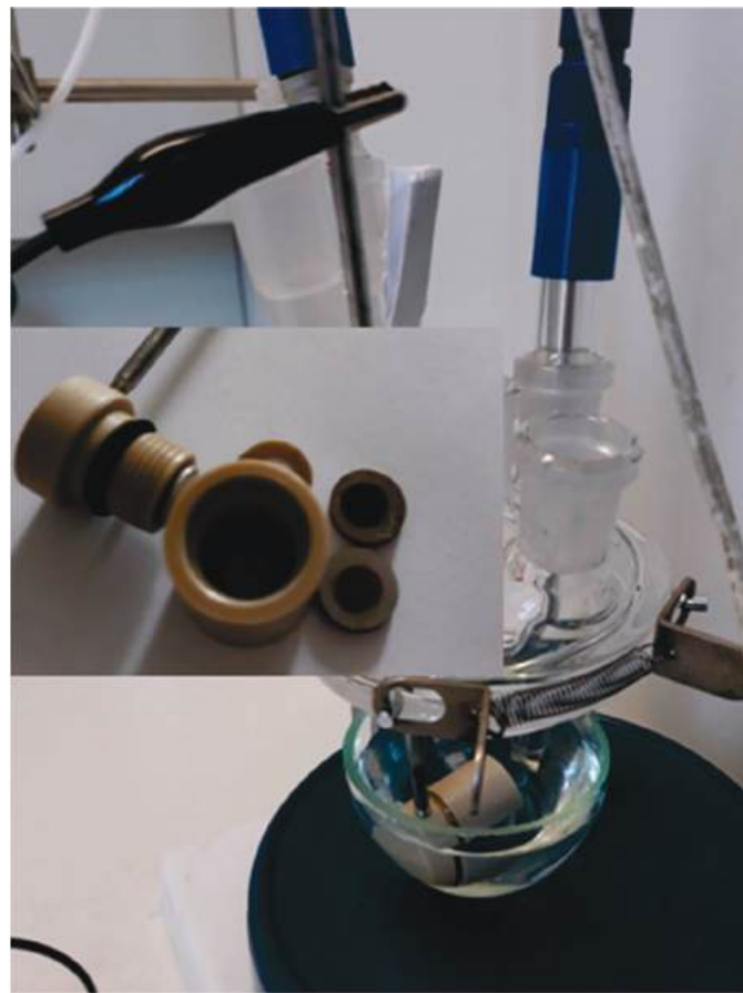
Figure 2. Electrochemical cell and disk work electrode.
