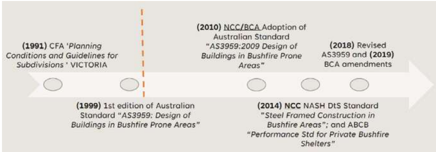
Figure 9.2 Timeline of the formal development of bushfire building standards in Australia (the dashed orange line indicates Year 2000)
