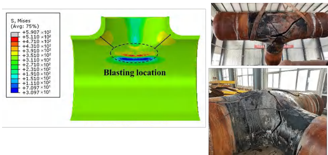
Figure 21. Simulated prediction and experimental verification of the blasting location for the SSES repaired low-strength tee.
