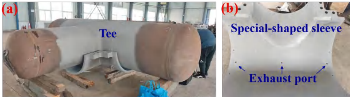
Figure 6. Surface cleaning and sand-blasting: (a) low-strength tee, and (b) special-shaped sleeve.
