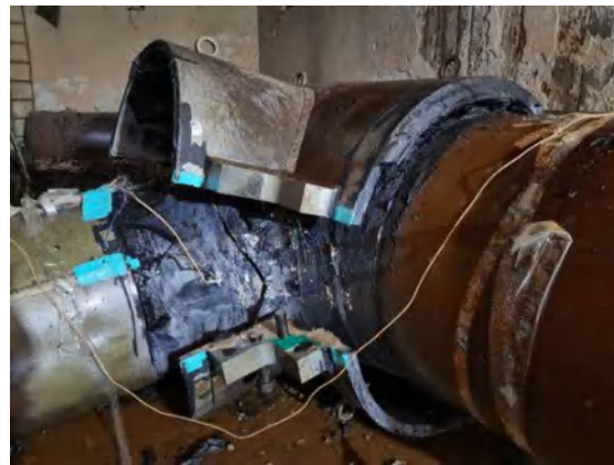
Figure 19. Failure of SSESS with bolt fracture.
