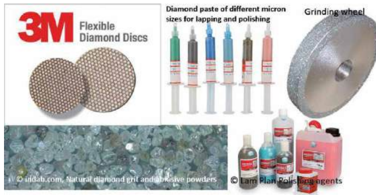
Figure 6. Diamond abrasive application.
