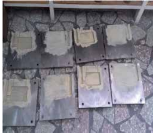
Figure 2. Metallic molds for casting Al_{0.8}CrFeCoNi alloy.
