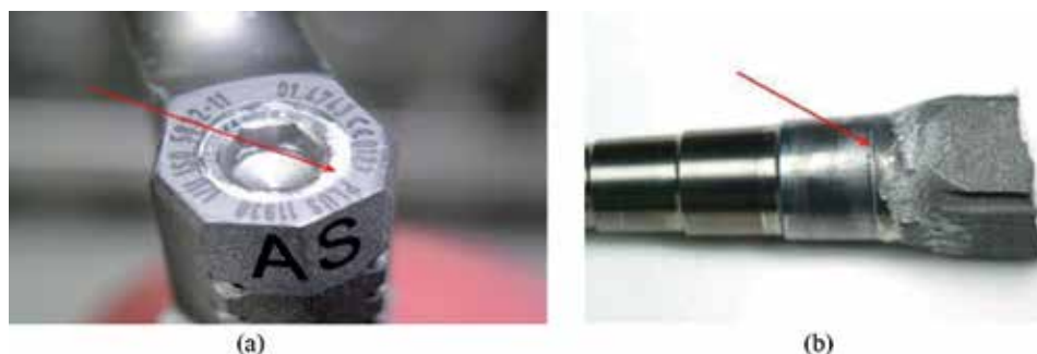
Figure 8. Sample #3. (a) Salt deposition in sample #3 and (b) crack of the distal module of sample #3.
