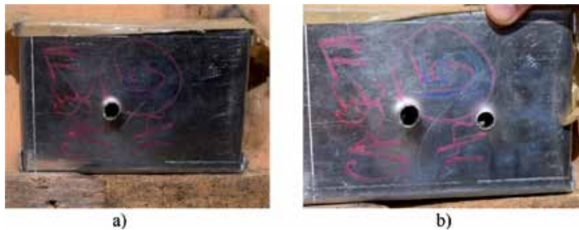
Figure 19. HEA-polymer ballistic package during dynamic tests. (a) after the first firing and (b) after the second firing.
