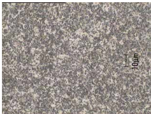
Figure 3. Microstructure of DF2 (AISI-O1) steel.
