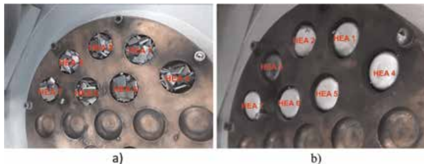
Figure 1. HEAB 1 to HEAB 7 batches prepared for melting on the copper plate of the RAV equipment (a) and after melting (b).
