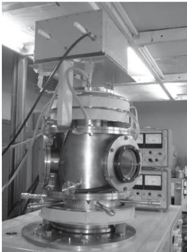
Figure 14. General view of the discharge chamber of an ion-plasma device [2].
