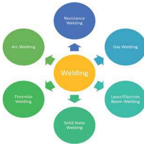
Figure 2. Various types of welding processes according to the temperature of the application.
