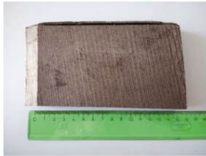
Figure 1. Illustrative cross-section from VVER-440 RPV (Original not-irradiated piece from VVER-440 V-213 RPV—Greifswald Unit 7).
