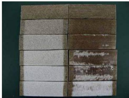
**Figure 5.** Discoloration of uncapped WPCs (left column) and Co-WPCs (right column) after various weathering times (0, 192, 432, 744, 1392, and 1952 h) [4].
