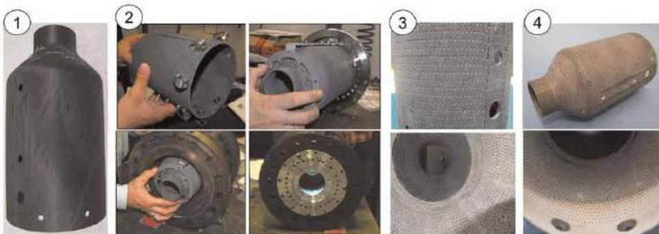
**Figure 8.** Oxide/oxide combustor liner developed by German Aerospace Center [15]. ① Oxide/oxide combustor liner for component test. ② Fit check with the oxide/oxide combustor liner. ③ Before the test. ④ After the test.
