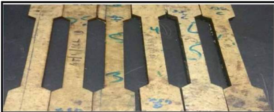
Figure 10. Specimen size for composite sheet material.
