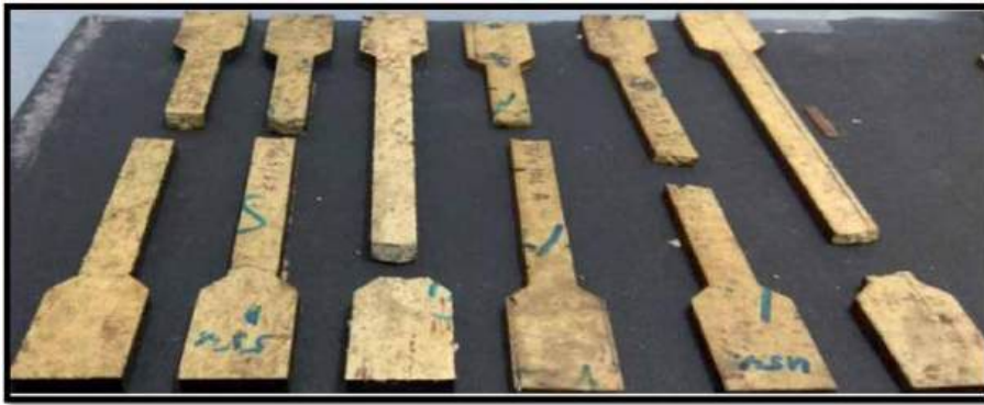
Figure 11. Specimen break after tensile strength test for composite material.
