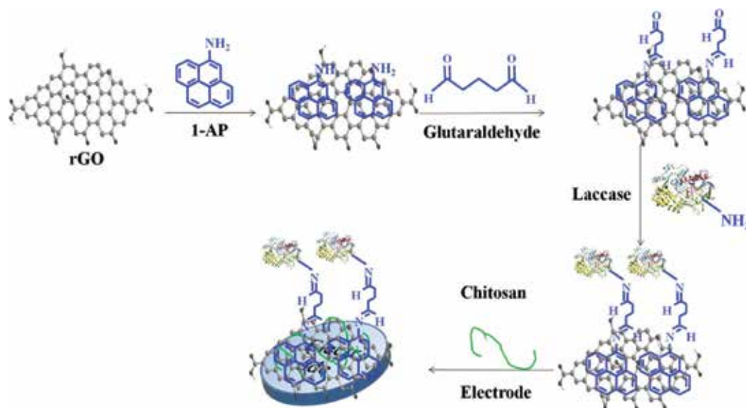
Figure 14. The preparation scheme of AP-rGOs/chitosan/laccase biosensor [23].
