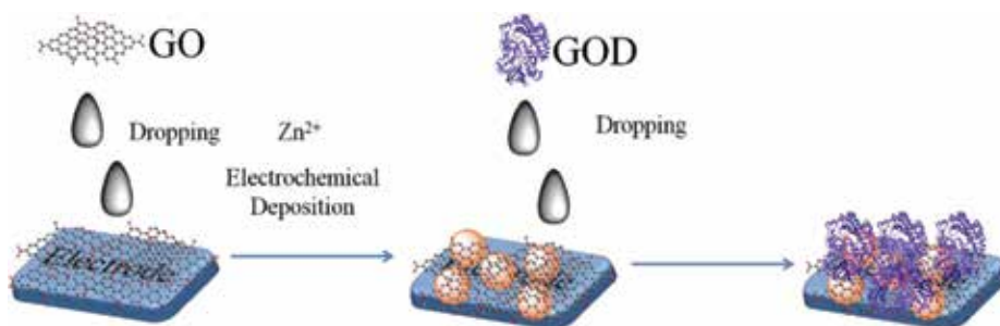
Figure 5. The preparation scheme of ZnO/GO/GOD-based glucose biosensor [11].
