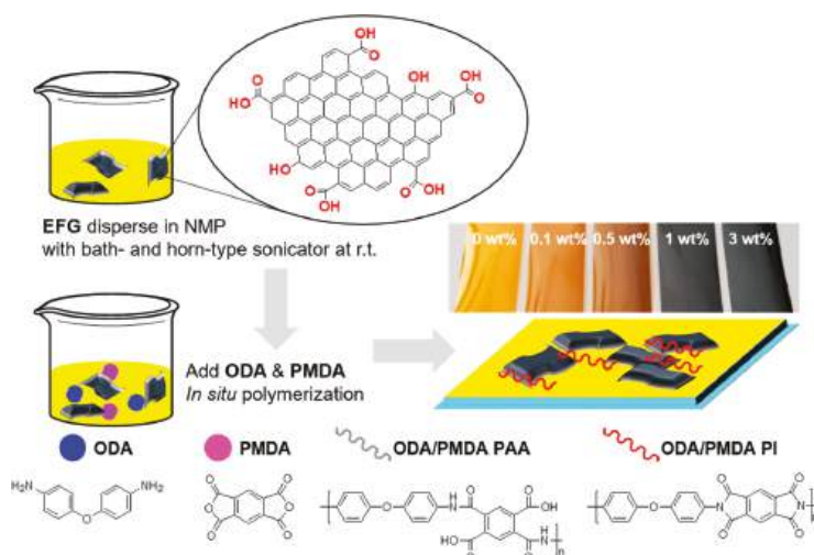
Figure 3. Fabrication process of PI/EFG composites.
