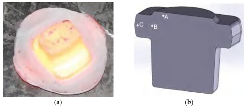
Figure 6. The flange forged on hammer (a), the flange model with areas of metallographic investigations marked (b). A, B, C – areas of metallographic observations on the forged part cross-section.
