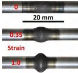
Figure 2. The shape of the samples after dilatometric testing—details of the heated central part.
