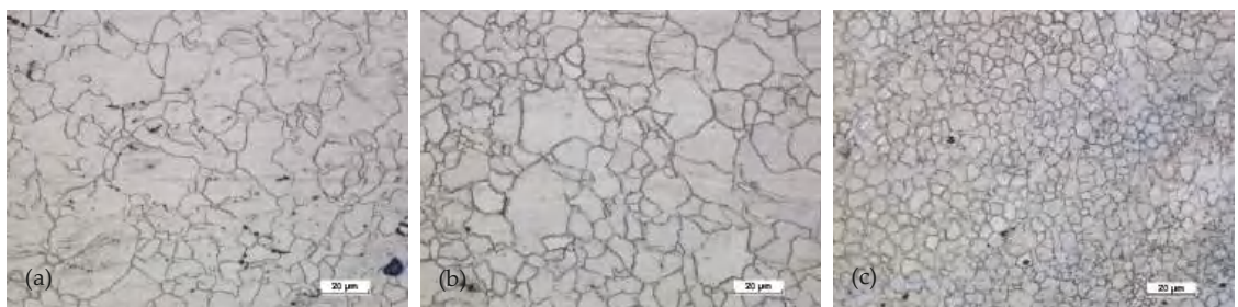
Figure 23. Microstructure for the forging obtained from the preform II: (a) first area of analysis marked on Figure 8, (b) second area of analysis marked on Figure 8, (c) third area of analysis marked on Figure 8.
