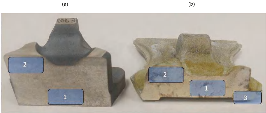
Figure 8. Microstructure test areas, (a) preform, (b) forging.
