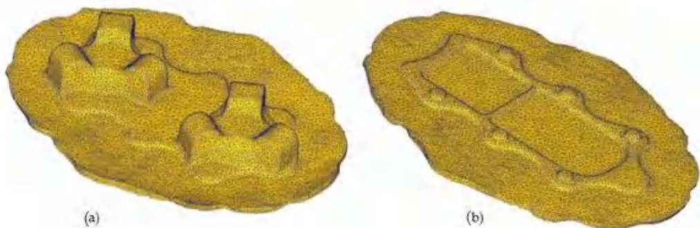
Figure 9. FEM-simulated shape of aircraft bracket forging: (a) top, (b) bottom.
