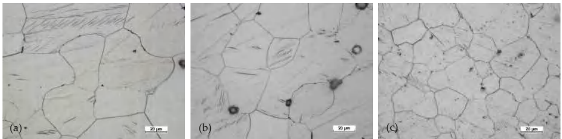
Figure 24. Microstructure for the forging obtained from preform I after forging and heat treatment: (a) first area of analysis marked on Figure 8, (b) second area of analysis marked on Figure 8, (c) third area of analysis marked on Figure 8.
