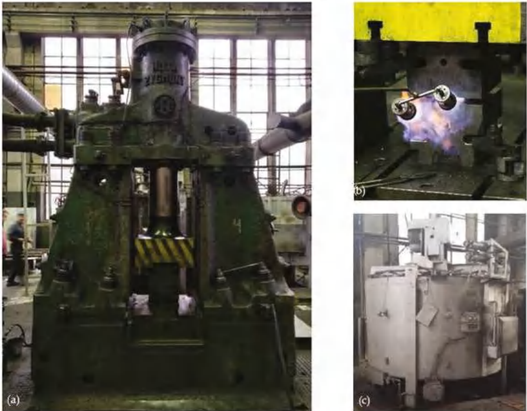
Figure 6. Machines used during tests in industrial conditions: (a) MPM 3150 drop hammer, (b) gas burner, (c) electric furnace.
