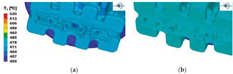
Figure 9. Temperature distribution—Al 6082 alloy: (a) punch feed speed 3 mm/s; (b) punch feed speed 6 mm/s.
