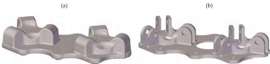
Figure 1. 3D models of the forging of aircraft mount from AZ61 alloy (a) and of the finished aircraft mount (b).
