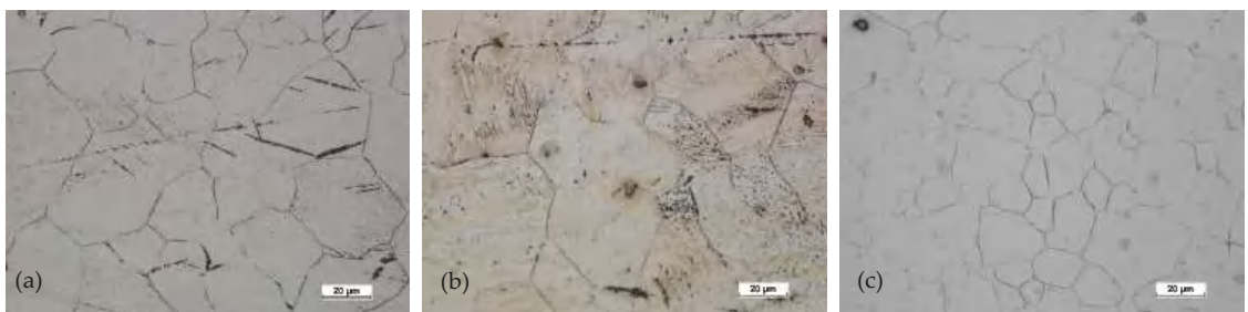
Figure 25. Microstructure for the forging obtained from preform II after forging and heat treatment: (a) first area of analysis marked on Figure 8, (b) second area of analysis marked on Figure 8, (c) third area of analysis marked on Figure 8.
