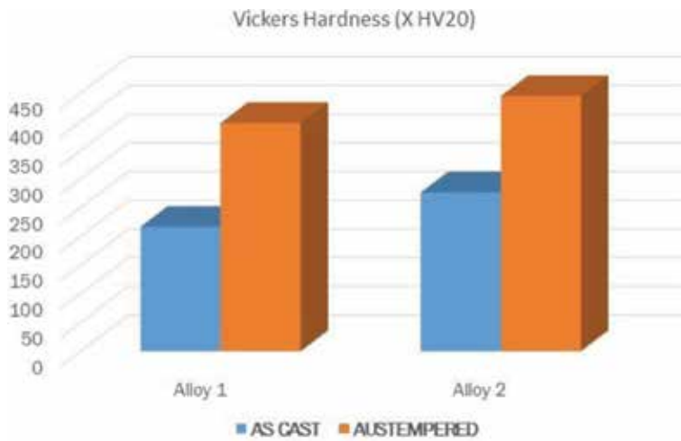
Figure 9. Vickers hardness for respective as-cast and austempered specimen.
