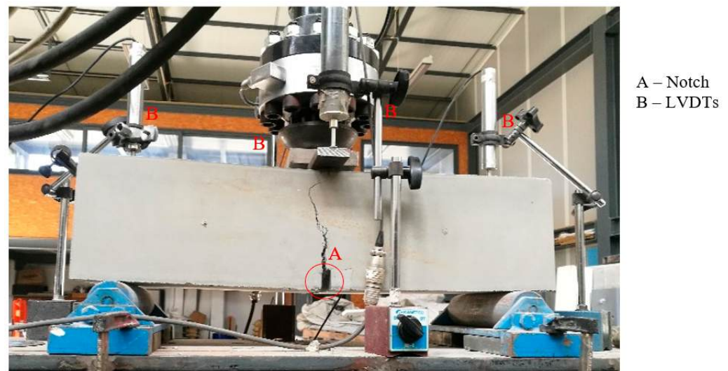
Figure 2. Test set-up and instrumentation.
