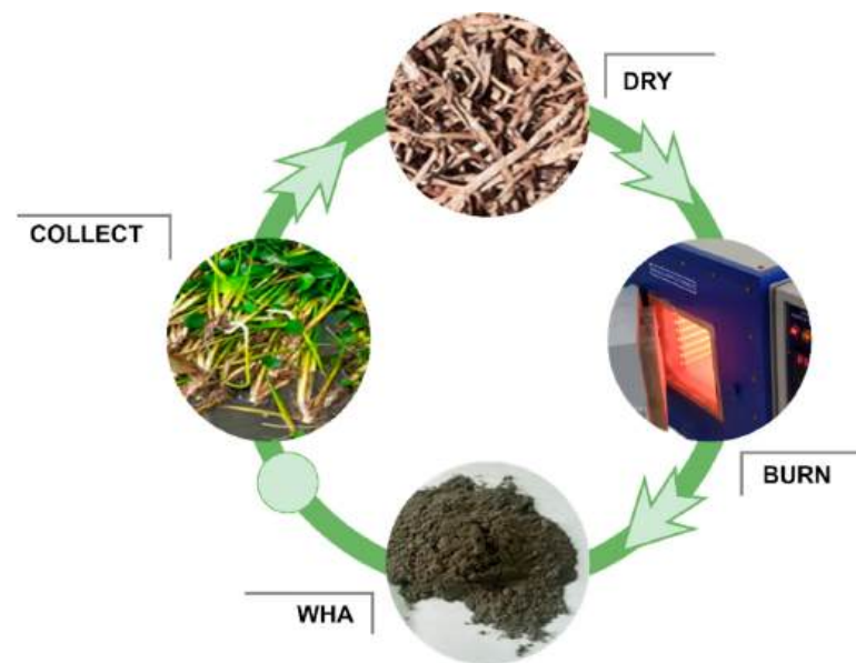
Figure 2. Main steps of the WHA production process.
