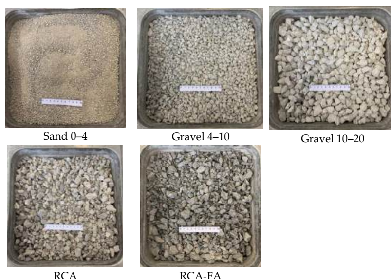
Figure 1. The raw and recycled aggregates (each line in the ruler is 1 cm).
