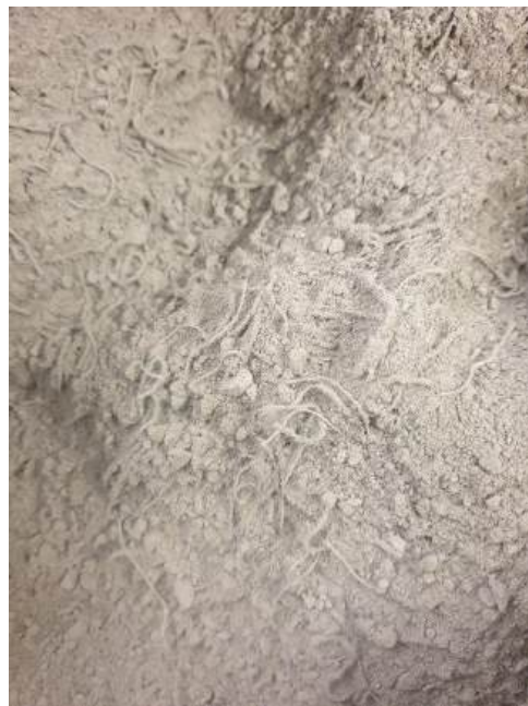
Figure 4. Dry mixture with cotton fibres.
