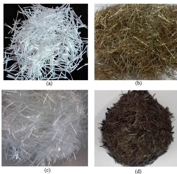
Figure 1. Fibers used in the formulation of eco-UHDC: (a) polymeric fibers, (b) steel fibers, (c) glass fibers, and (d) basalt fibers.
