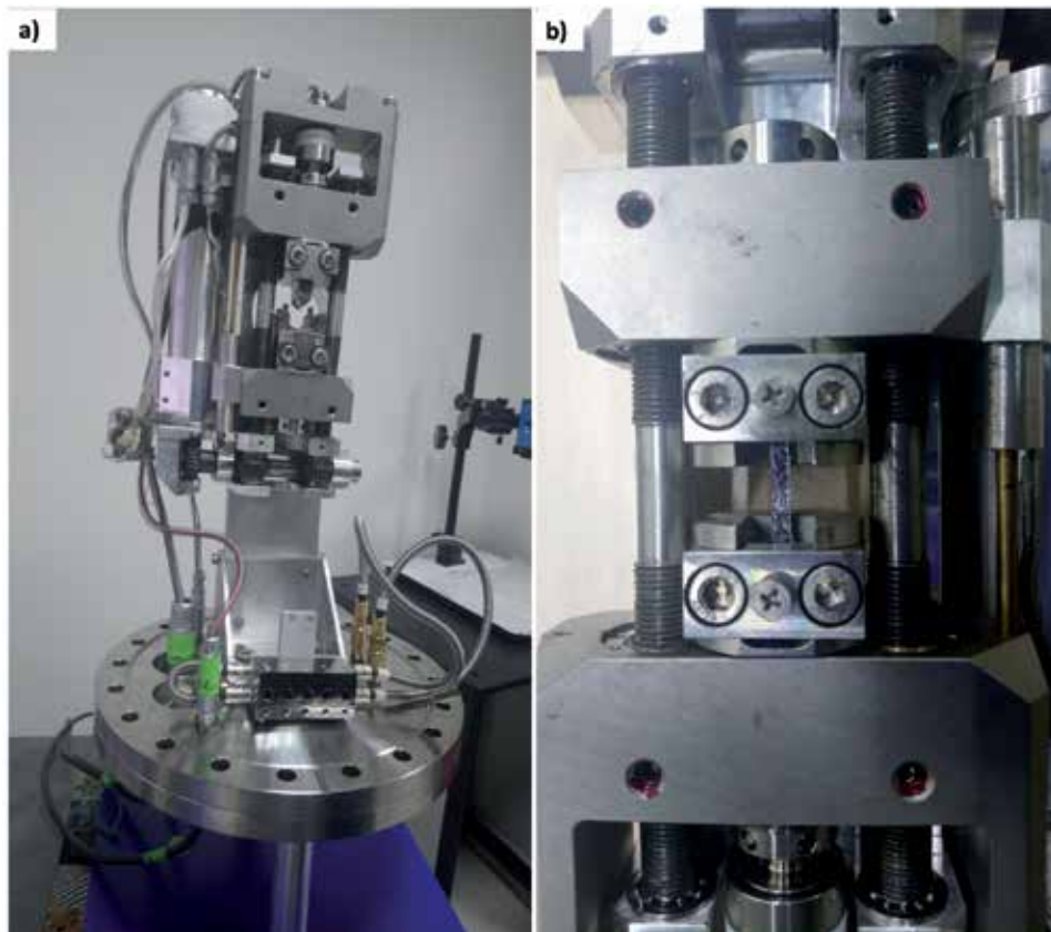
Figure 6. Microtensile test module mounted in the vacuum chamber base (a) and detail of the test section with a probe (b).
