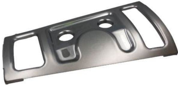
Fig. 20.2 Exemplary application part (inspection door Airbus A320), produced with the process combination of stretch forming and incremental sheet forming
