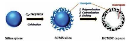
Figure 4. Typical synthetic scheme for HCMSC capsule [33] (copyright (2010) American Chemical Society).
