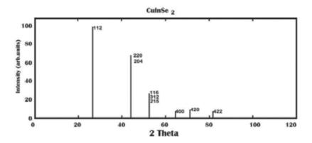
**Figure 11.** Simulated XRD spectra of non-stoichiometric CuInSe2; Cu:In:Se2 = 0.21:0.26:0.53.
