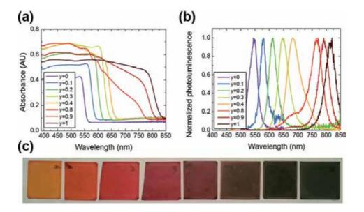
**Figure 3.** (a) UV-Vis absorbance spectra of FAPbI $_y$ Br $_{3-y}$  metal-halide perovskite films with different y values. (b) Steady-state photoluminescence spectra for the corresponding films. (c) Photographs of the films with y increasing from 0 to 1 (left to right). Reproduced with permission from Ref. [30]. Copyright 2014, Royal Society of Chemistry.
