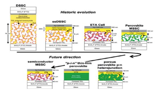
**Figure 2.** Historic evolution of the solar cell technology, starting from the electrolyte-based mesoscopic DSSC, the ssDSSC, the ETA cell to the MSSC perovskite absorber and the n-type TiO<sub>2</sub> reprinted with permission from ACS [17].
