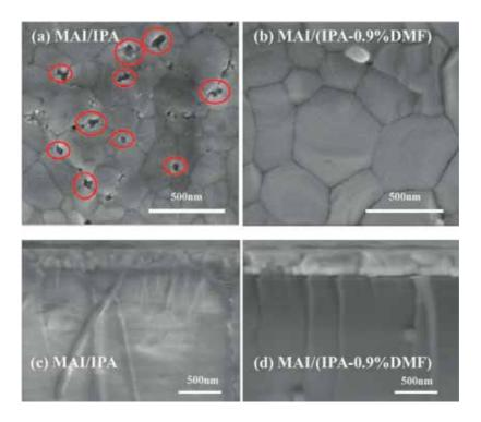
Figure 8. SEM images of perovskite films. Higher-magnification SEM image of the perovskite film without (a) and with  $(b) DMF \ additive, cross-sectional \ SEM \ image \ of \ the \ perovskite \ film \ without \ DMF \ additive \ (c) \ and \ with \ (d) \ DMF \ additive \ (d) \$ (reprinted with the permission from [31], 2017, the Royal Society of Chemistry).
