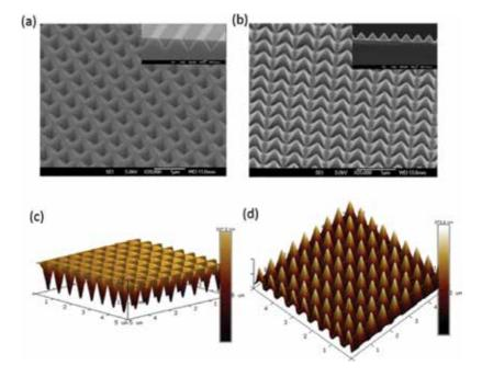
**Figure 2.** 30°-tilted view SEM images of (a) inverted nanopyramid Si master mold and (b) upright nanopyramid structured on the glass, and the inset images are the cross-sectional views of SEM images. Three-dimensional AFM images (c) inverted nanopyramid Si master mold and (d) upright nanopyramid structured glass.
