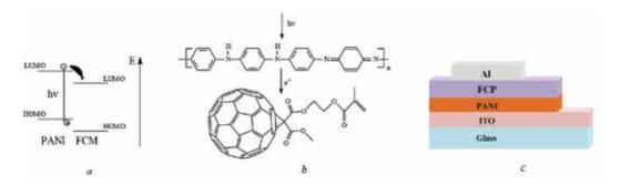
**Figure 6.** (a) An energy level diagram of the PANI/FCM system; (b) process of photon absorption and charge separation in this structure; (c) multilayer film structure of OSC.
