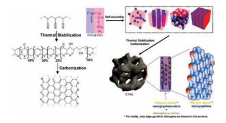
Figure 6. Schematic representation of preparation of CTNC [42] (copyright (2015) Royal Society of Chemistry).
