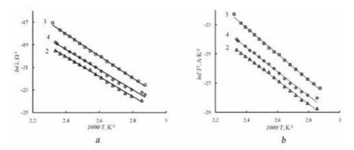
**Figure 5.** Dependences of (a) the electrical conductance and (b) I/T<sup>2</sup> on the inverse temperature for films of copolymers (o-toluidine with 2-(1-methyl-2-buten-1-yl)aniline) in different molar ratios: (2) 1:3, (3) 1:1, and (4) 3:1.
