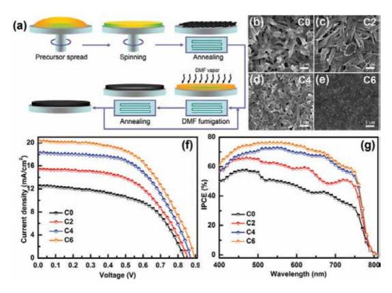
**Figure 6.** (a) Schematic processing procedure for MAPbI<sub>3</sub> film deposition (C0) and recrystallization *via* DMF vapor fumigation for 2 (C2), 4 (C4), and 6 (C6) cycles. (b–e) Surficial SEM images of samples C0, C2, C4, and C6. (f) J-V curves and (g) IPCE spectra of the devices based on samples of C0, C2, C4, and C6, respectively. Reproduced with permission from Ref. [45]. Copyright 2015, Royal Society of Chemistry.
