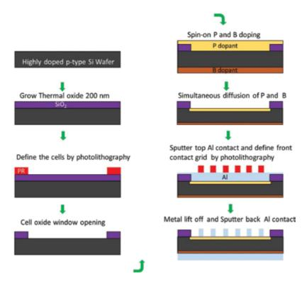
Figure 3. The schematic representation of monocrystalline Si solar cell fabrication process.
