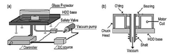
Figure 7. Schematic representation of a home-built spin coater (a) and details of the rotor (b) [33].
