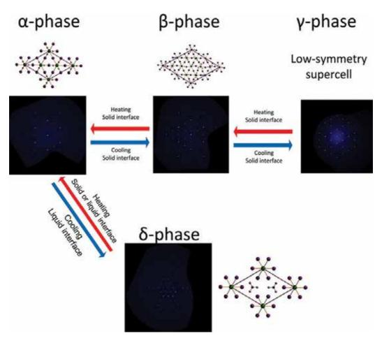
Figure 2. Graphical scheme of phase transitions of MA(Pb,Sn)X<sub>3</sub> materials. Precession images are drawn at [006] view. Reproduced with permission from Ref. [24]. Copyright 2013, American Chemical Society.
