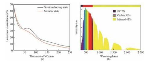
**Figure 2.** (a) Calculated luminous transmittance for single-layer VO<sub>2</sub> films with various thickness at semiconducting state (black line) and metallic state (red line) and (b) the solar spectrum and relative energy distribution.
