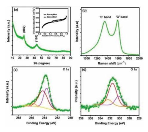
Figure 9. (a) XRD pattern, (b) Raman spectrum, and (c-d) XPS spectra of the HPC sample. The inset of (a) shows the nitrogen adsorption–desorption isotherm of the HPC sample [29] (copyright (2017) Elsevier).
