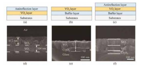
Figure 3. Schematic illustration of VO,-based films with (a) antireflection layer, (b) buffer layer, and (c) both of antireflection layer and buffer, respectively. Relative SEM images of three typical structures have been shown in figures. (d)–(f) corresponding to figures. (a)–(c) [12, 33, 72], respectively.
