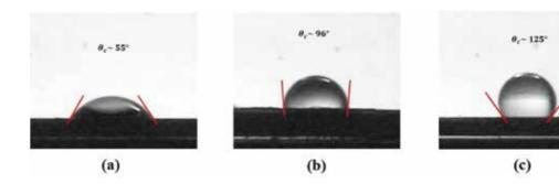
**Figure 14.** Photographs of a water droplet on: (a) planar solar cell, (b) patterned solar cell with nanopyramids and (c) SAM-coated patterned solar cell.  $\theta$  c is the water contact angle.
