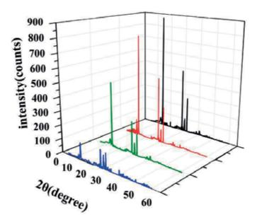
**Figure 3.** XRD patterns of CH3NH3PbI3 films with pristine (blue), IPA/DMSO vapor (green), IPA vapor (red), and IPA/DMF vapor (black) annealing (reprinted with the permission from [24], 2016, Elsevier).
