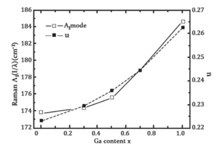
Figure 13. Room temperature Raman shift in CuIn<sub>1</sub>-xGaxSe<sub>2</sub> thin-films of thickness 600 nm deposited on a glass substrate with a change in Ga content, the Raman peak shifted from 173.8 to 184.6 cm<sup>-1</sup> in A1 mode and u is Se shift parameter. Reproduced with permission.
