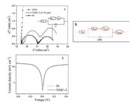
**Figure 11.** (a) Nyquist plots of the symmetric cells consisting of FTO glass, NMC-3, and Pt electrodes, respectively, equivalent circuit element for Pt CE in the inset. (b) Equivalent circuit element for NMC-3 porous carbon. (c) Tafel polarization curves of the symmetric cells fabricated with two identical Pt and NMC-3 electrodes [35] (copyright (2013) Elsevier).
