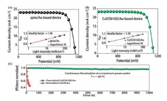
**Figure 5.** PV measurements of PSC based on spiro-OMeTAD and CuSCN HTM. (A) JV curve for the spiro-OMeTAD based device. (B) J-V curve for the CuSCN-based device. (C) Operational stability of an unencapsulated CuSCN-based device with and without a thin layer of reduced graphene oxide (rGO), reprinted with permission from Science [58].
