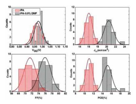
**Figure 13.** Comparison of histograms of photovoltaic parameters for the perovskite solar cells based on MAI/IPA (red) and MAI/(IPA-0.9%DMF) (black) condition. Data from 20 cells were used for the histogram (reprinted with the permission from [31], 2017, the Royal Society of Chemistry).
