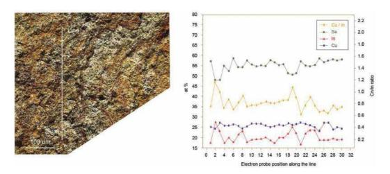
Figure 2. Chemical composition of a near-stoichiometric CuInSe2 film measured consecutively by using an electron beam with a 3 nm probe size along a line marked on a TEM micrograph (left) and the plotted data (right) (corresponding to the data in Table 1).
