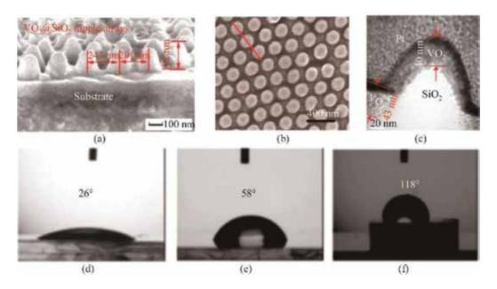
**Figure 8.** (a) SEM cross-sectional profile of the sample with 210 nm period, (b) top-view SEM image of the sample with 440 nm period, (c) TEM cross-sectional image to show the thickness of  $VO_2$  coatings on  $SiO_2$ , (d) planar  $VO_2$ , 210 nm patterned  $VO_2$  with 40 nm thickness, and 210 nm patterned  $VO_2$  with fluorooctyl triethoxysilane (FOS) overcoat.
