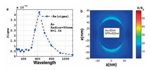
**Figure 5.** (a) Wavelength-dependent extinction spectra. (b) Electric field distribution of gold metal nanoparticle of radius 50 nm embedded in silica matrix.
