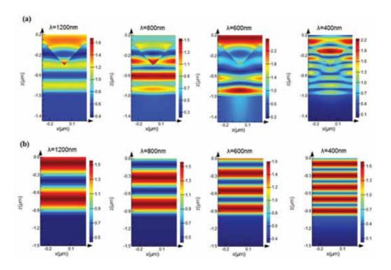
**Figure 12.** The cross-sectional electric field distribution profiles at different wavelengths employing FDTD analysis (a) INP coated Si with a period of 600 nm, the base size of 500 nm and depth of 400 nm and (b) planar Si subjected to same light conditions.
