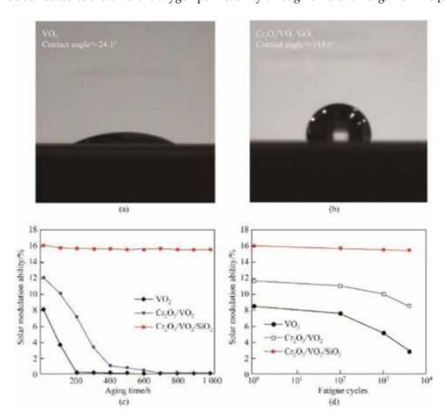
**Figure 6.** Images of contact angle measurement of (a) the single-layer VO<sub>2</sub> and (b) the proposed  $Cr_2O_3/VO_2/SiO_2$  structure. Variation curves of  $\Delta T_{sol}$  for VO<sub>2</sub>,  $Cr_2O_3/VO_2$ , and  $Cr_2O_3/VO_2/SiO_2$  with different duration time (c) and different fatigue cycles (d).
