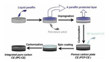
**Figure 5.** The fabrication procedure of the integrated pure carbon counter electrode for DSSCs [34] (copyright (2013) Royal Society of Chemistry).
