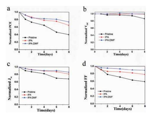
**Figure 6.** Stability of the devices with the structure of ITO/PEDOT:PSS/perovskite/PCBM/Ag: (a) normalized PCE, (b) normalized VOC, (c) normalized JSC, and (d) normalized FF (reprinted with the permission from [24], 2016, Elsevier).
