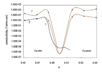
$\textbf{Figure 4.} \ \ \text{The measured conductivity of the CuInSe}_2 \ \text{thin-film along the Cu}_2 \\ \text{Se-In}_2 \\ \text{Se}_3 \\ \text{on-tie line with composition (Cu}_2 \\ \text{Se)}$  $1-x(In_2Se_3)x(Iine\ 1)$  and the calculated range (between line 2 and 3) near the  $Cu_2Se_1In_2Se_3$  tie line at 300 K.
