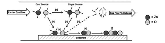
Figure 6. ZnO thin film fabrication. Mechanism with CVD [32].
