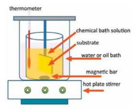
Figure 3. The arrangement of CBD equipment [16].
