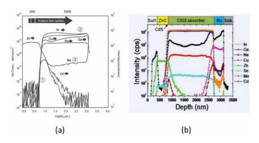
Figure 7. SIMS depth profile of Cu, In, Ga, Se, Cd, and Na. (1) CdS/CIGS and ZnO diffusion. (2) Cu, In, Ga, and Se depth profile. (3) Quantitative analysis of Na in CIGS.
