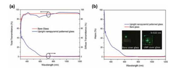
**Figure 4.** (a) Measured total and diffuse transmittance spectra of the bare glass and the UNP patterned glass as a function of wavelength and (b) the optical haze spectra of the bare glass and the UNP patterned glass as a function of wavelength. Photographs of diffracted light patterns of the corresponding samples obtained from the green diode laser with a wavelength of 532 nm are also displayed in the inset.
