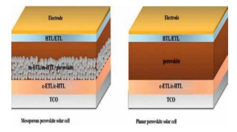
**Figure 3.** Schematic illustration of perovskite solar cells architectures, c-ETL; compact electron transporting layer, c-HTL; compact hole transport layer, m; mesoporous, TCO; transparent conductive oxide.
