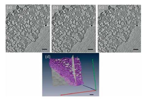
Figure 2. Panels (a), (b), and (c) represent three longitudinal slices extracted from the volume reconstruction of the PSiNW nanostructures revealing an area of highly porous medium. The bare scale is 50 nm. (d) 3D tomography TEM image of nanowires [32].
