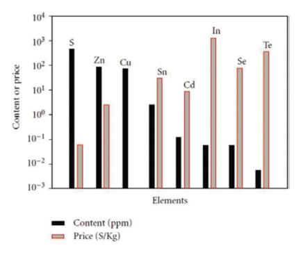
$\textbf{Figure 16.} \ \ \text{Content and the world trading price of the elements used in light absorbers CdTe, Cu}_2ZnSnS_4, \ \text{and } CuInSe_2 \ \text{for } SnS_4, \ \text{and } SnS_4, \ \text{a$ thin film solar cells.
