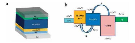
Figure 4. (a) Schematic structure of the devices in this study: ITO/PEDOT:PSS/CH<sub>3</sub>NH<sub>3</sub>PbI<sub>3</sub>/PCBM/Ag. The thickness of each layer was not in scale with the real thickness for clarity. (b) Schematic illustration of energy band diagram of studied devices (reprinted with the permission from [24], 2016, Elsevier).
