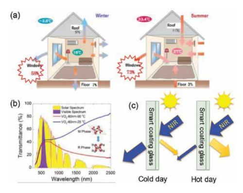
**Figure 1.** (a) Schematic of energy exchange in winter and summer days. (b) Typical optical properties of thermochromic coatings before and after phase-transition temperature. Inset is the crystallographic structure of  $VO_2$  (monoclinic phase) and  $VO_2$  (rutile phase). (c) Schematic of energy-efficiency based on thermochromic smart coatings.
