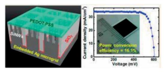
Figure 8. Embedded metal electrode for highly efficient organic-inorganic hybrid nanowire solar cells, and I-V characteristic of the solar cell [52].
