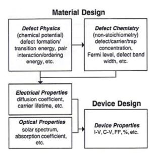
**Figure 1.** The scheme of our materials design and device design in which the electrical and device properties are optimized, and related to the process parameters such as, chemical potential and non-stoichiometry.
