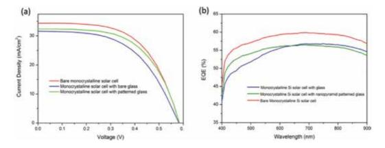
**Figure 7.** (a) Current density-voltage characteristics and (b) external quantum efficiency (EQE) spectra of encapsulated monocrystalline Si solar cell with and without the upright nanopyramid patterned cover glass and bare cover glass.
