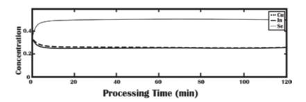
Figure 10. The Se or H<sub>2</sub>Se RTP of Cu:In:Se = 0.24:0.25:0.51 CuxIny films at  $450^{\circ}$ C,  $\mu$ Cu = 0,  $\mu$ In = 0; the mole ratio of the constitute atoms (in the film) as functions of the processing time (120 min). (Film volume = (2.5 cm)  $2 \times 2 \mu$ m).
