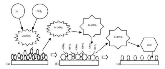
Figure 4. Mechanism of ZnO thin film growth [21].
