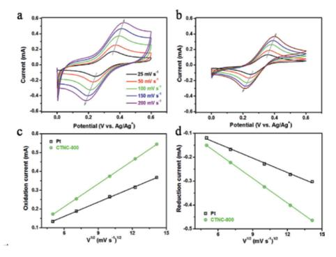
**Figure 12.** Cyclic voltammograms using CTNC-800 (a) and Pt (b) cathodes in with various scanning rates. The oxidation (c) and reduction (d) peak currents with respect to the square root of scanning rate [42]. Copyright (2015) Royal Society of Chemistry.
