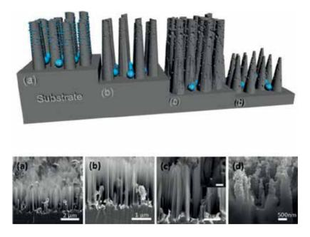
**Figure 3.** (a-i)–(d-i) The schematic illustration of the proposed qualitative etching model for the formation of PSiNWs using Ag-assisted HF/H<sub>2</sub>O<sub>2</sub> electroless etching technique. (a-ii)–(d-ii) The corresponding SEM micrographs, prepared using various HF concentrations [33].
