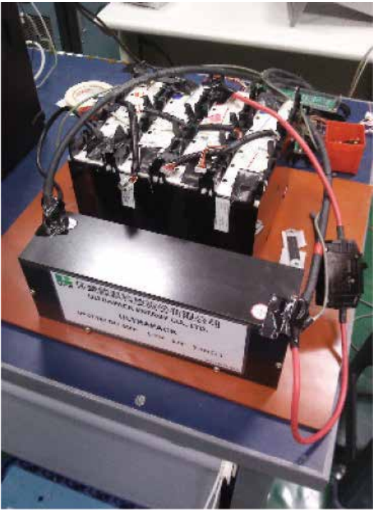
Figure 12. Implementation of RLIB with EMS and auxiliary physical battery (left: EMU; Central: LiFePO 4 LIB pack; and right: auxiliary physical battery).
