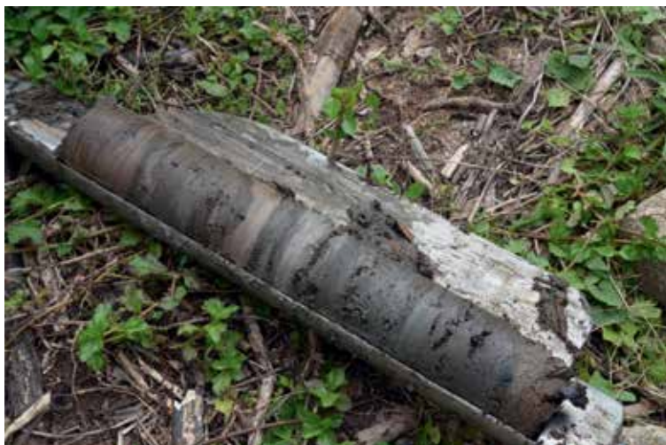
Figure 5. Sediment core collected from mangrove ecosystem to study the metal proxy and sediment accumulation rate. Photo by Ong Meng Chuan.
