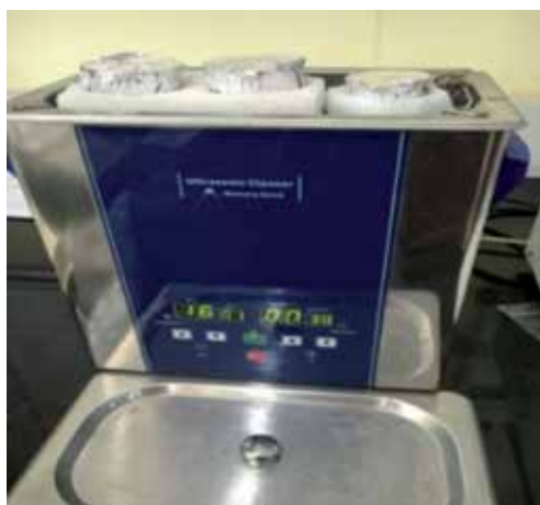
Figure 14. Actual setup of CS/PMMA homogeneous solution by magnetic stirrer and ultrasonication.
