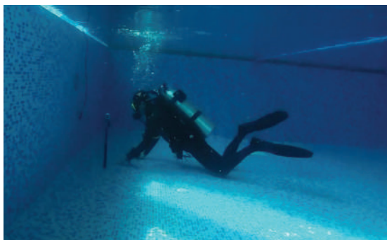
Figure 4. In experiment, one channel data acquisition system is used to record the diver's breathing sound underwater. Sample rate is 50 kHz.
