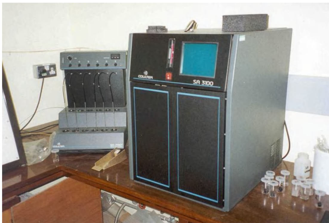
Fig. 8.1 COULTER-3100 for measuring the BET surface area for dust particles
